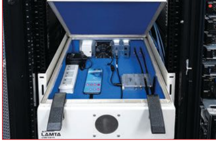
▲ Fig. 2 LAA4 Compact 4-channel attenuator array inside an RF shield box.
